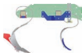
Spring loaded ridging body with bed loosening tines 2 (height adjustable)
