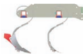
Ridging body with leaf spring tines 5 (fitted direct to the front frame)
