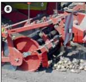
Windrow intake for light soil with centre share and rubber roller or for heavy soils with rotor shaft
