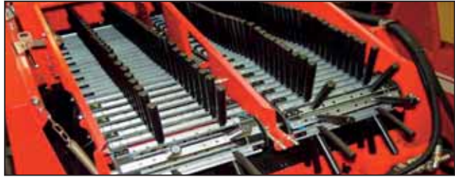
Type UB: best separation on cloddy soil with little stone content
