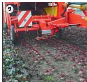
Vegetable intake: through typed share with support rollers. Special solutions are possible.
