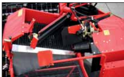
Type NB with 3 rd hedgehog web and 3 rd scraper roller – for increased output on soils with fewer clods
