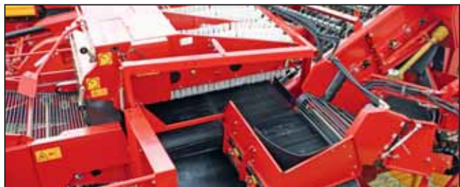
Type SB: best separation on stony soils with the innovative kinetic stone separator
