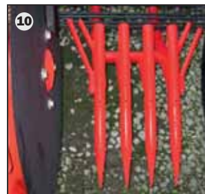
Carrot intake: large, distance adjustable support wheels, manual depth adjustment and a 1- or 2-row carrot share. Various row width and distances possible
