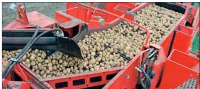
Type NB: best separation on soils with little clods and trash
