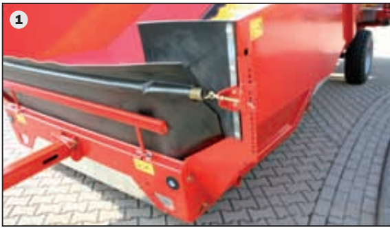
1 Simple: simple height adjustment to suit different trailers in steps with the spring loaded intake flap
