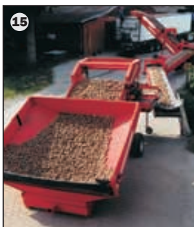
11 Simple solution: electrically operated "left/off/right" flow direction of the cross conveyor – optimum control via operator terminal
