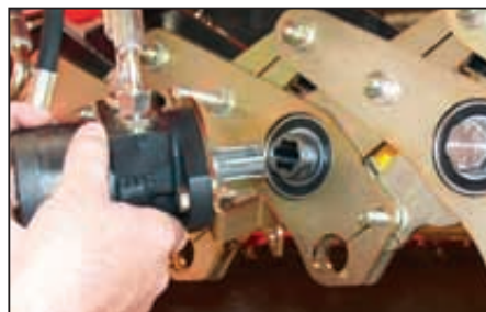
Direct connected: direct drive of the rollers in place of traditional high maintenance chain drives!
