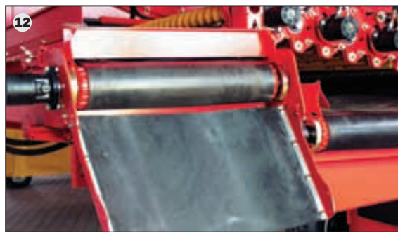
12 Reduced drop: Flow brake reduces the drop speed for gentle delivery into boxes.
