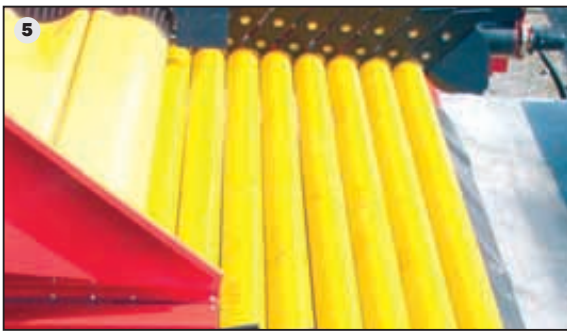
5 Increase your cleaning: two additional pre-cleaning rollers
