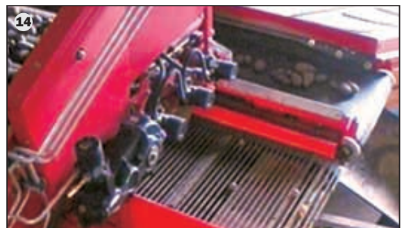
14 More separation: main web – in lieu of a cross conveyor – to separate small potatoes from soil
