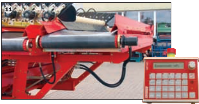
11 Simple solution: electrically operated "left/off/right" flow direction of the cross conveyor – optimum control via operator terminal
