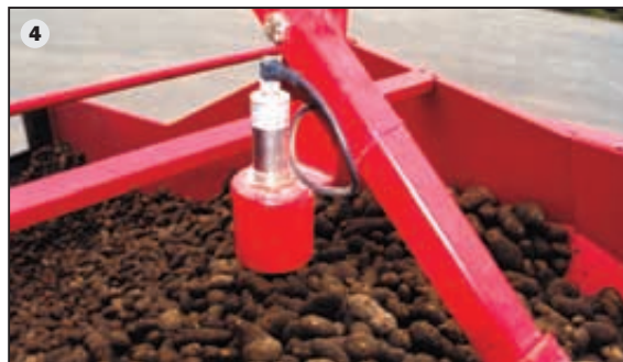
4 Successful system: CAPACITY-CONTROL-system (option) automatically controls the hopper belt speed and ensures an optimum crop flow through the whole line. You're advantage: even flow without manual changes. Controlled via ultra-sonic sensors
