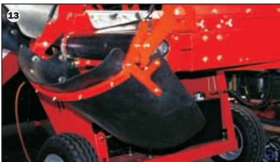
13 Less drop: gas cylinder operated chute to reduce the drops dramatically and even more gentle box filling
