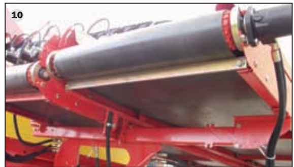
10 More reach: cross conveyor extension from 300 cm to 350 cm
