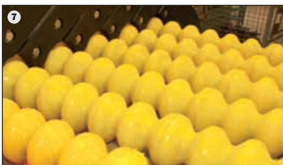
7 Good separation: special polyurethane pre-grading rollers for high output and gentle pre-grading. Gap adjustment is possible according to the required grading size.
