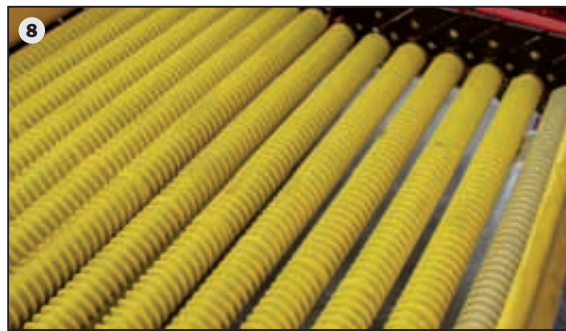
8 For best separation and grading results: with up to 14 polyurethane rollers for an effective and gentle pre-grading as well as high cleaning with highest gentle crop handling, also under heavy conditions
