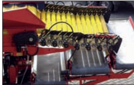
Clean crop: the standard hydraulic levelling and gap adjustment – for optimum cleaning of the crop
