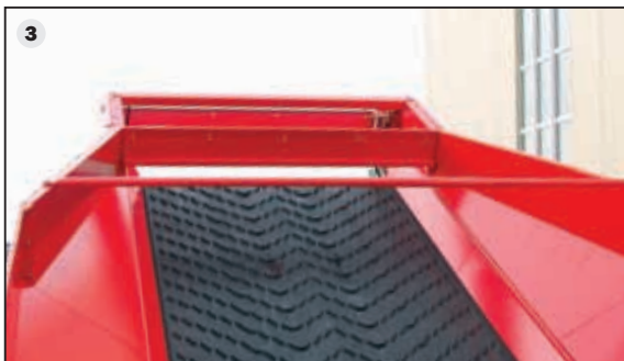
3 Even flow: The hopper retaining wall ensures even crop flow and a consistent feed to the following machines.
