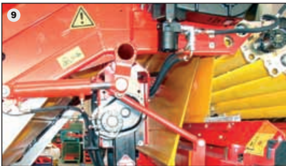
9 More flexible: hydraulic gap and levelling adjustment for flexible and simple adaptation to suit individual storing conditions
