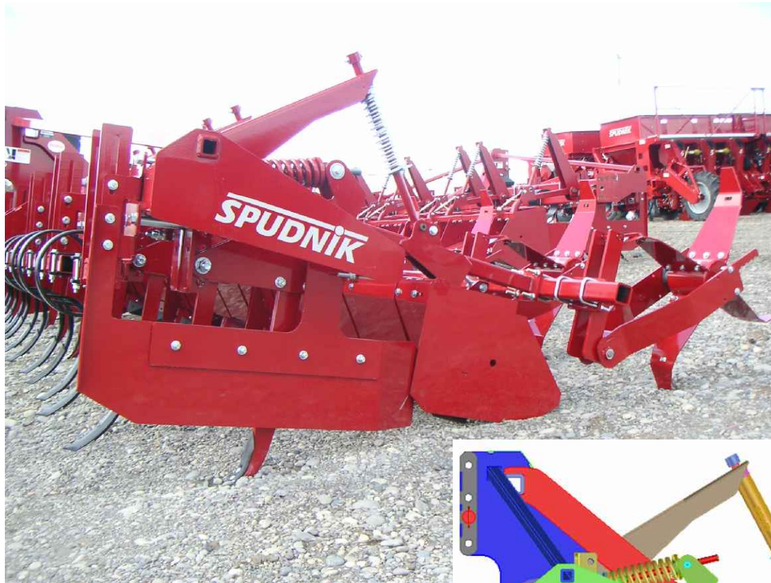
SPUDNIK Prop with Former Heavy ripper shanks Light S-Tines in front
