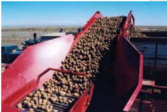
5. Continuous operation reduces maintenance costs due to stop/starts and greatly reduces bruising
