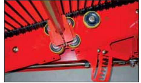
Mechanical rotary agitator (hydraulic adjustment available as option)
