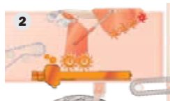
... or only the front element of the TwinSep is lowered: The crop flows over only half of the RS separator.
