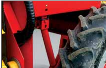
Automatic levelling (option) Always in balance: Automatic levelling during harvest is another option for working on hillside location.
