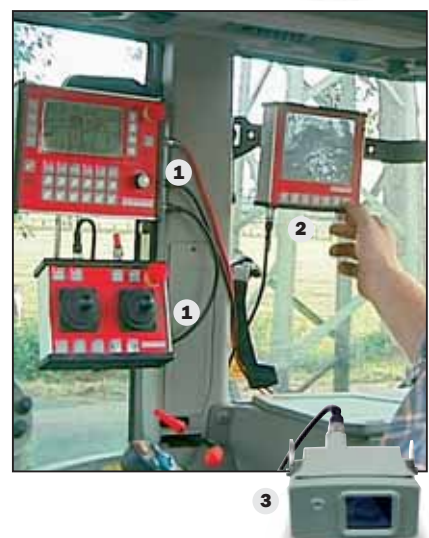
Monitor (option) Useful visual aid: with two cameras (3) and one monitor (2) do not miss anything during digging
