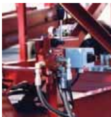
Quick and simple height adjustment of the elevator when you are unloading without using pups.
